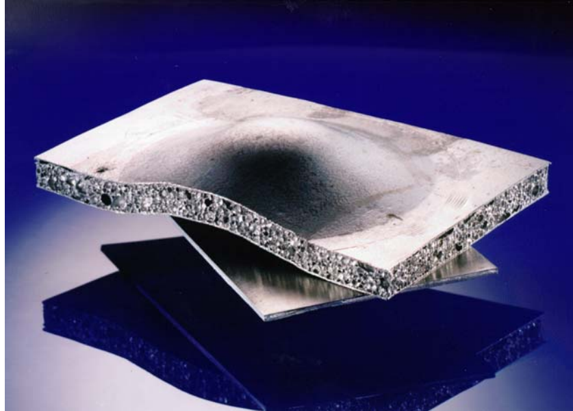
Fig. 14: Aluminium foam sandwich (foamed and unfoamed, steel face sheets)
